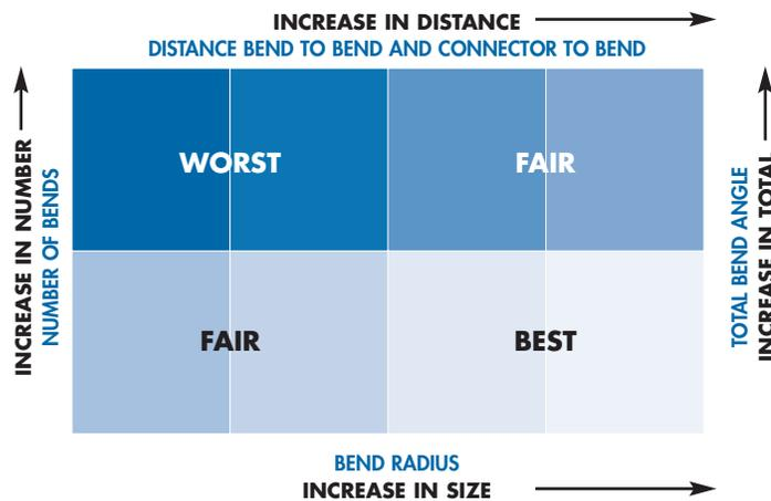
*NOTE: Minimum bend radii listed in this catalog are the absolute minimums recommended, based solely on mechanical considerations.*
