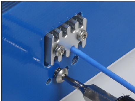
From back face of PC board, loosen and remove 2 retention screws from daughter card assembly bracket.
